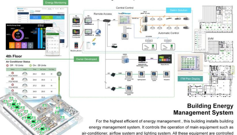
and handled by Daikin product (Intelligent Touch Manager) and Monitoring software is installed to monitor and verify the result of energy saving as designed.
